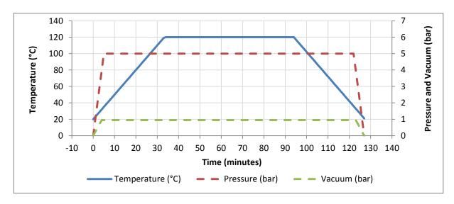
HexPly<sup>®</sup> M10R is a flexible curing system and can be cured at temperatures from 85 to 150°C, at pressure between 0.9 to 5 bar. Heat up rate can be also adapted (from 0.5 up to 10°C/min) depending the part design.
